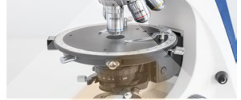
Center-adjustable and turnable polarisation stage
