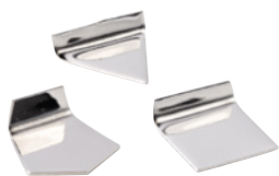
Milligram weights, flat polygonal sheet
