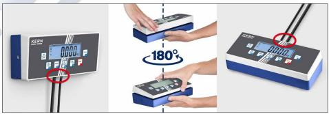
■ Verification plug, for verified balances this enables you to separate the display device and platform without affecting the verification, e.g. for installing the scale in a packing and dispatch table, pit frame etc. at a later date. Please order this at the same time as you purchase your scale, see accessories
