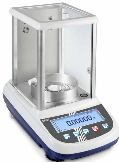
**KERN ALJ 200-5DA with optional ioniser** see accessories. High-precision semi-micro analytical balance. Thanks to its high level of precision, it is ideal for calibrating pipettes
