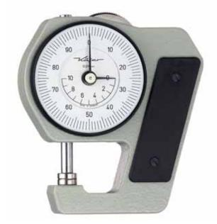
The contact points are in contact when the Pocket Dial Thickness Gauges J 12 and J 15 are not in use. The serrated lifting wheel opens them for the insertion of the component. The size can be easily read off the scale. The instruments can be zeroed by using the knurled adjusting bezel.
