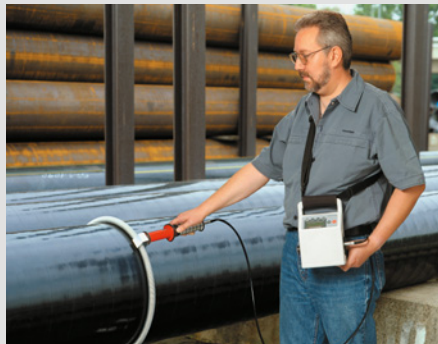
Porosity detection on pipelines
